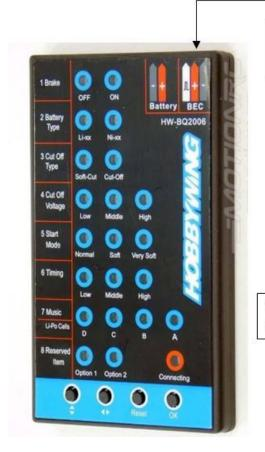
ESC connector plugs in here Apply battery power thru ESC, not direct to the battery connector on the card!
